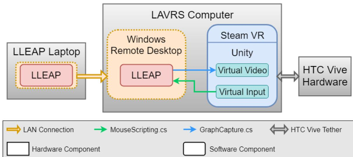
Figure 5.2: Graph showing the connections between the different hardware used.
