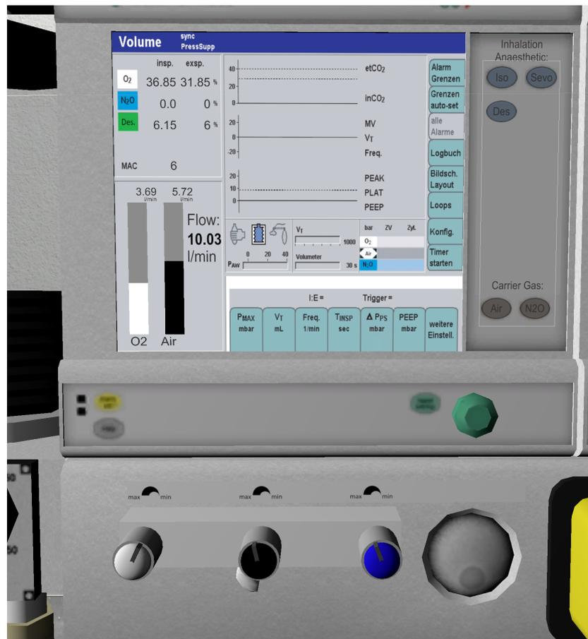
Figure 5.4: Screenshot of the respirator’s setting’s menu. At the very bottom are three knobs for adjustment of the flow of the different gas types (white: O<sub>2</sub>, black: carrier, blue: inhalation anesthetic). The monitor above shows the absolute flow values and concentrations in percent as well as the MAC. Right from the monitor buttons for the choice of inhalation anesthetic and carrier gas can be found.
